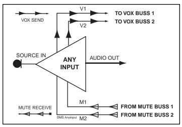
Fig. 8 - Any Input VOX and MUTE Functions
